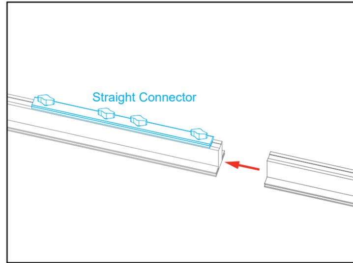
Slide connector across seam of extrusions.
