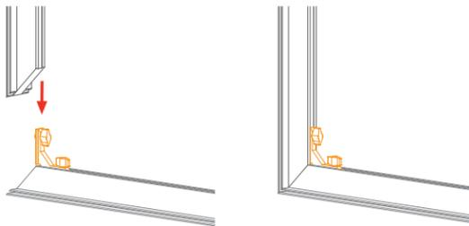
Keep corner connectors attached to horizontal extrusions.
