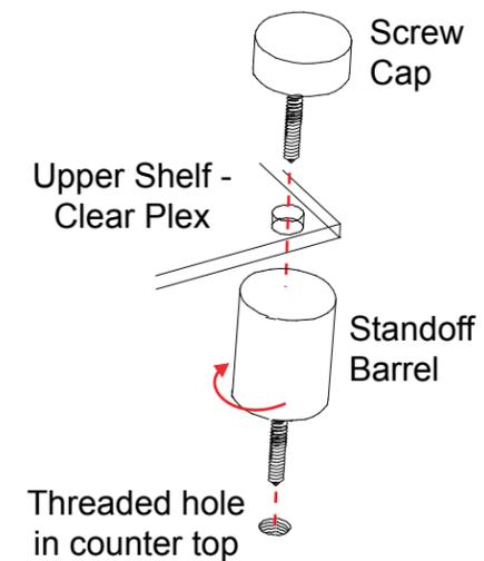
Attach standoff barrels to counter and secure in place. Secure upper shelf to standoffs using screw caps.
