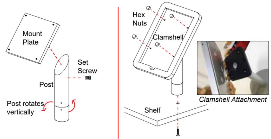
1. Attach Mount Plate to Post, using Set Screw.
