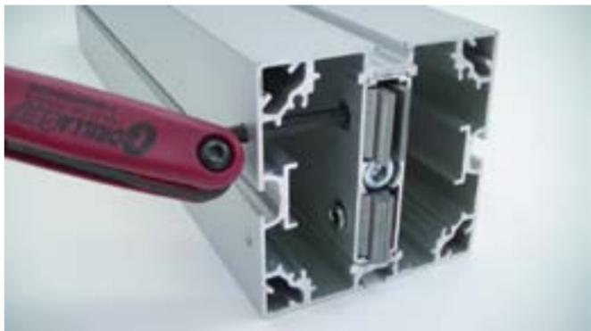
Turn the hex wrench clockwise to open the lock and secure in the groove.
