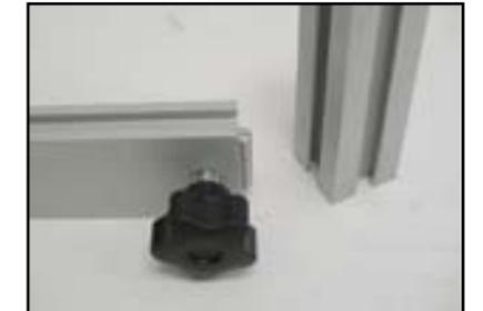
Detail F: Plastic Star Knobs are used to tighten locks where horizontal extrusions connect with vertical extrusions. Turn the knobs clockwise to tighten. Turn counter-clockwise to loosen, but do not remove knob. Do Not Overtighten.
