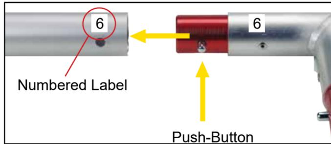
Connections are made by holding the button down and sliding the red tube until it locks in place. To disassemble, push button and pull or twist extrusions apart.
