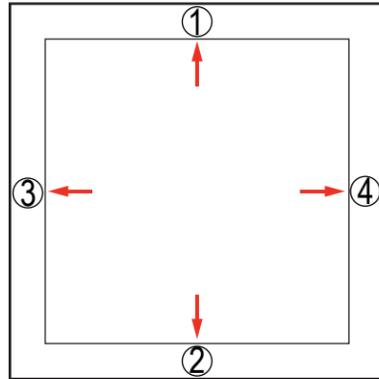
Once corners are attached, press the middle of edge 1 into the channel. Then press middle of edge 2 into the channel on opposite side.
