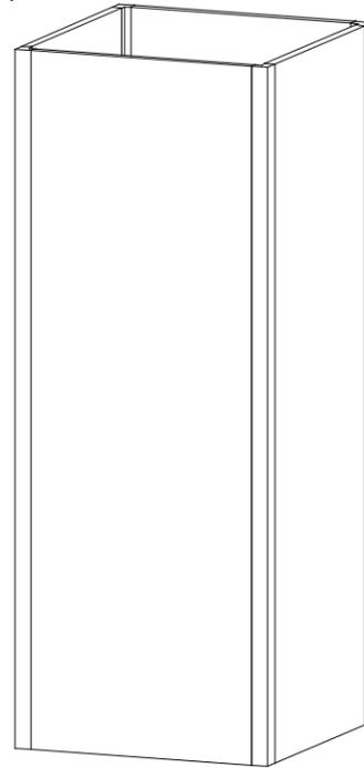
Attach panels in numerical order and set internal shelf on shelf supports.
